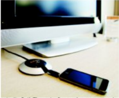
Audio Pull-Through: One end connects to the in-room TV and the other plugs into the headphone jack of any iPod, laptop, or MP3 player.
